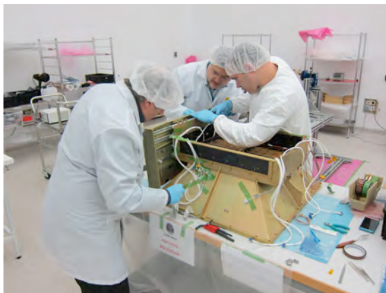
Structural Thermal Modell for ASIM
