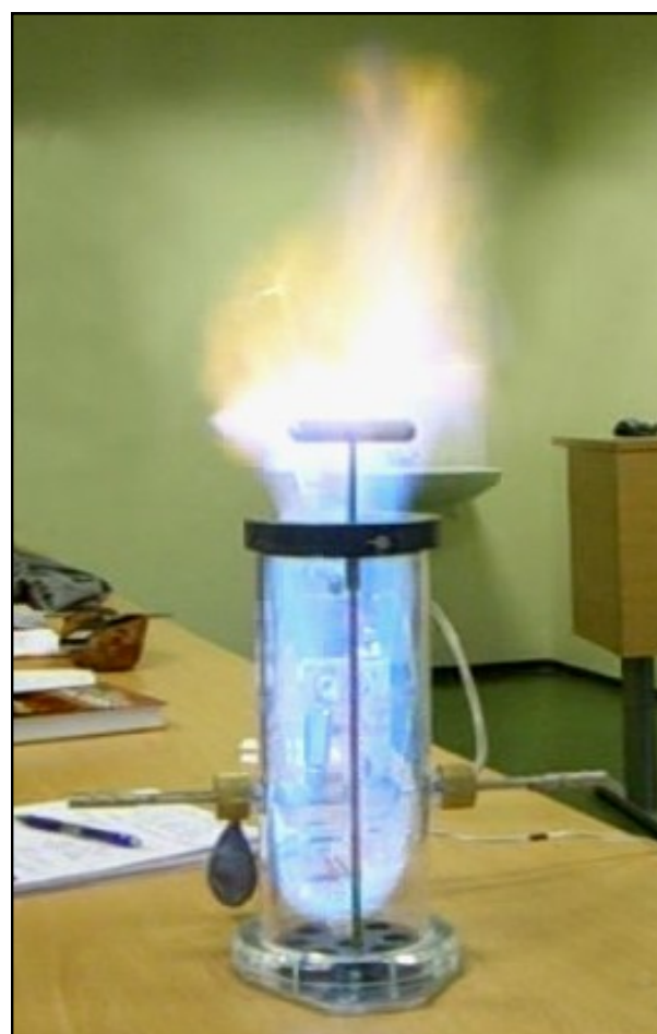
Photo of gas explosion in a 2-litre pyrex-container. Demonstration/exercise in the PTEK250 course: "Explosion Hazards in the Process Industries".
