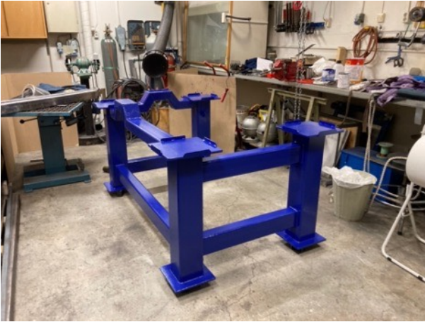
Thanks to the superb welding skills of Kris (Kristoffer Eikehaug) we now have a stable table frame for the nanoLace system.
