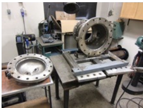
The picture above and below show the finished pipe and explosion chamber for the Process Technology group.
