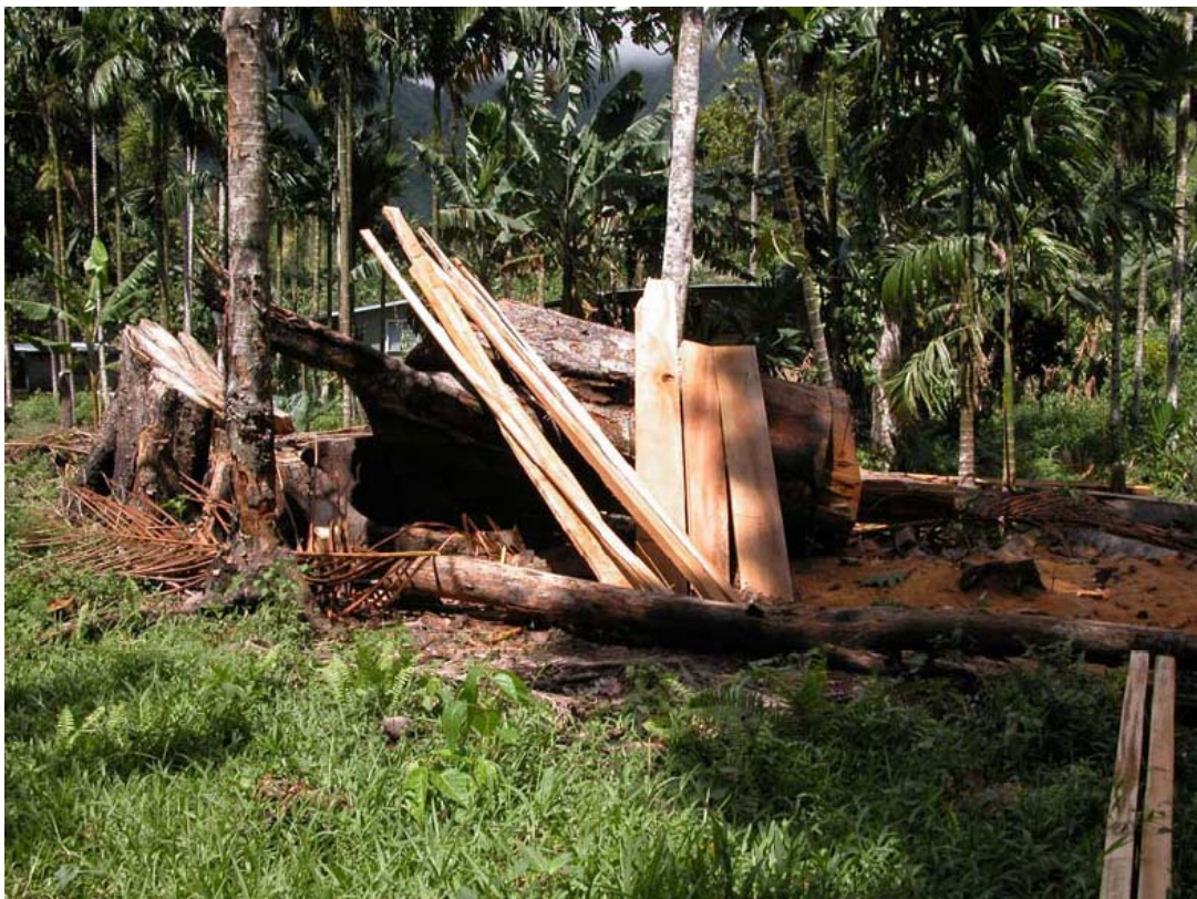
Figure 5. A recently felled and partly sawn breadfruit tree on Niolam Island (Lihir Group), the beams from which will be used as structural timbers in the construction of a local house.
