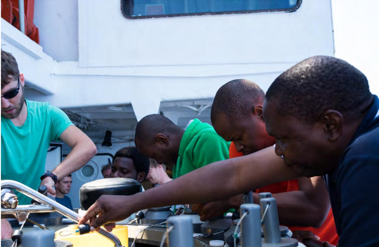
**Fig. 2:** Work at sea usually starts with a briefing for the different instrumentation used during the cruise, here it is the preparation of the CTD probe before the station work (Photo: SvN).
