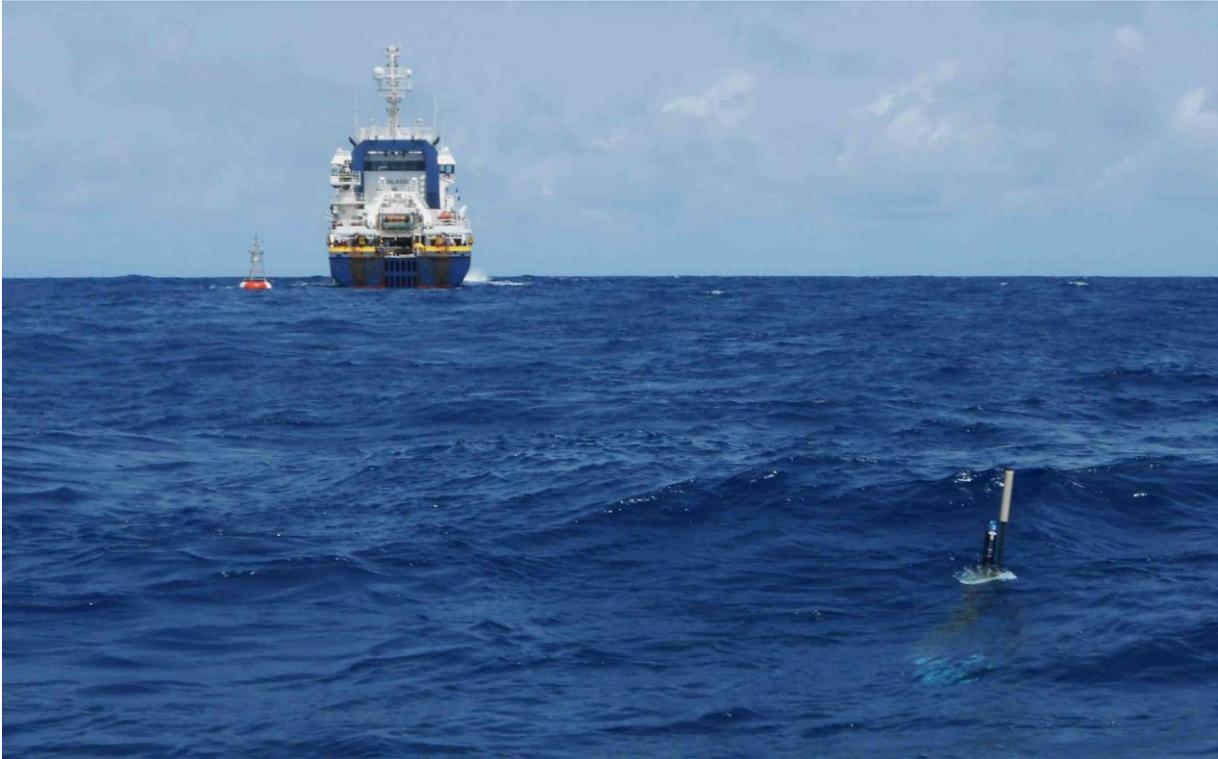
A Deep-Argo profiler just after its deployment at 10°W-0°N, close to the just serviced ATLAS buoy observed on the left of the R/V Thalassa (Courtesy: B.Bourlès, IRD).
